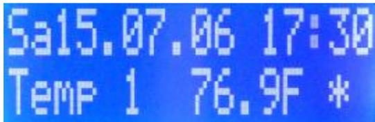
The cooling symbol (\*) is displayed, indicating that the controller has activated the relevant switchable socket (if present) to lower the temperature.
